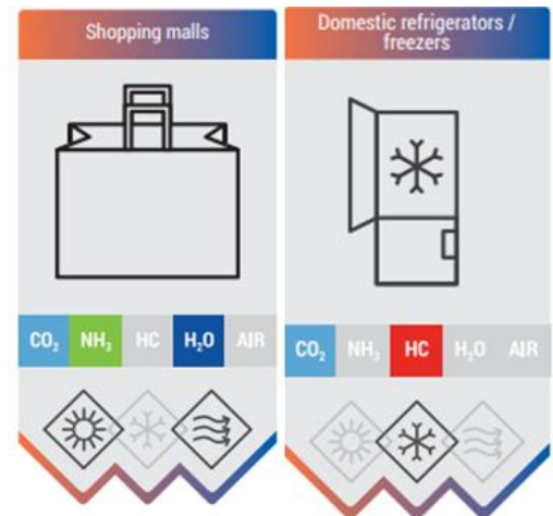
FIGURE 7 – NATURAL REFRIGERANT OPTIONS FOR APPLICATIONS
