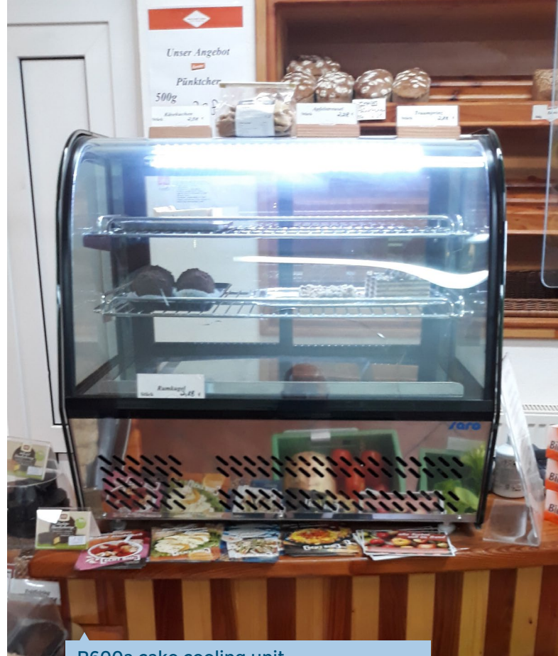
R600a cake cooling unit.
